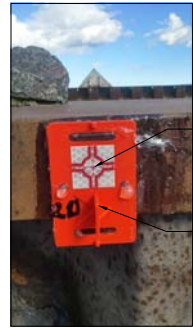
TYPICAL TARGET INSTALLATION
